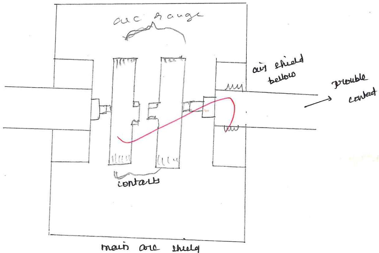
It consists of fixed contacts moving contacts and arc shield mounted inside a vacuum chamber the mounting member is connected to the control mechanism by stainless steel bellows. This enable the permanent sealing of the vacuum chamber of eliminate the possibility of leak.
