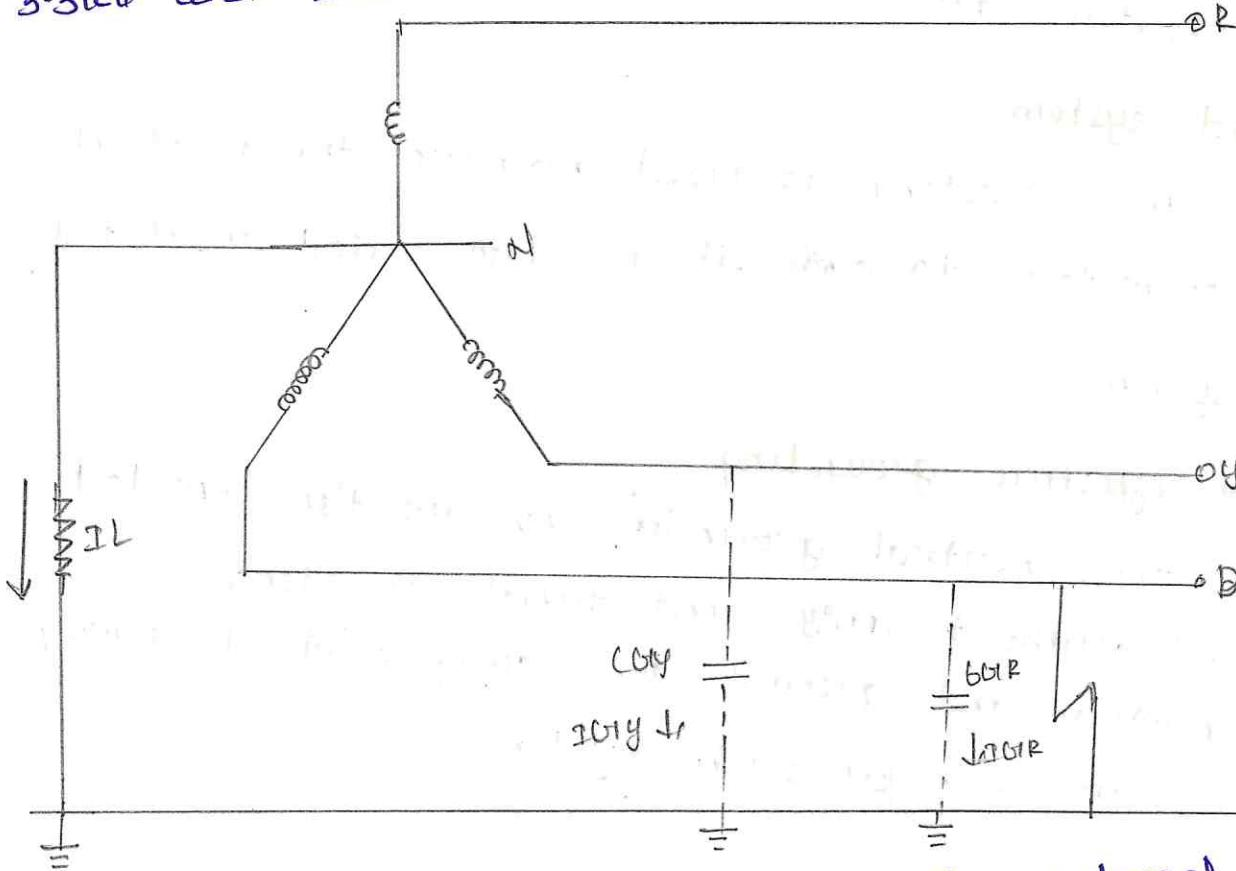
In the circuit below 3.3kV the external resistance in neutral circuit is unnecessary because the voltage available between line and earth is only 280V. If earth resistance is  $1.5\Omega$  then the each current is limited to  $280/1.5$ .
