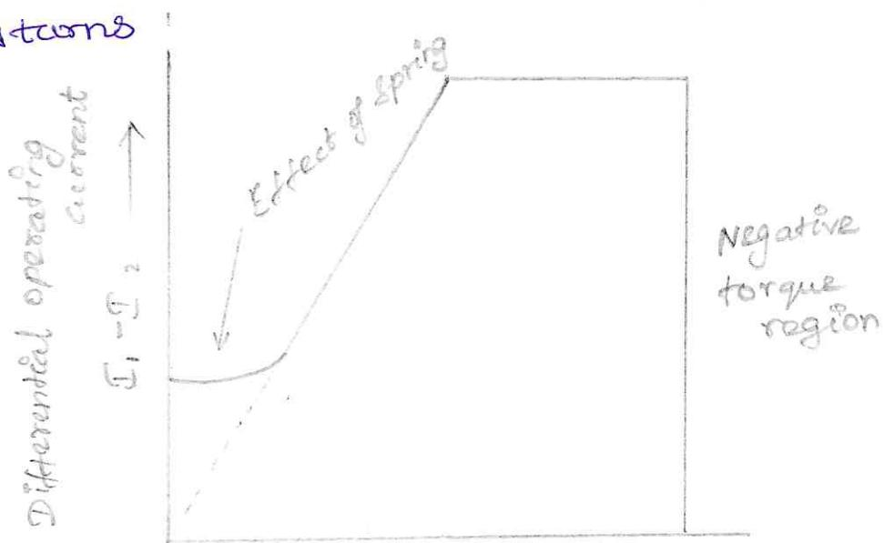
Settings of moving coil relay  $\frac{I_1 + I_2}{2}$  average restraining current  $\rightarrow$
