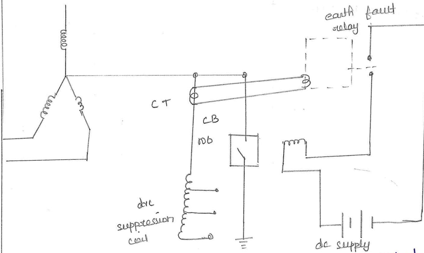
The coil is rated at continuous rated current equal to maximum earth fault current however if a speed earth fault occurs a circuit breaker closes after a certain time lag and the earth fault current flows through the parallel circuit by passing the dc suppression coil.
