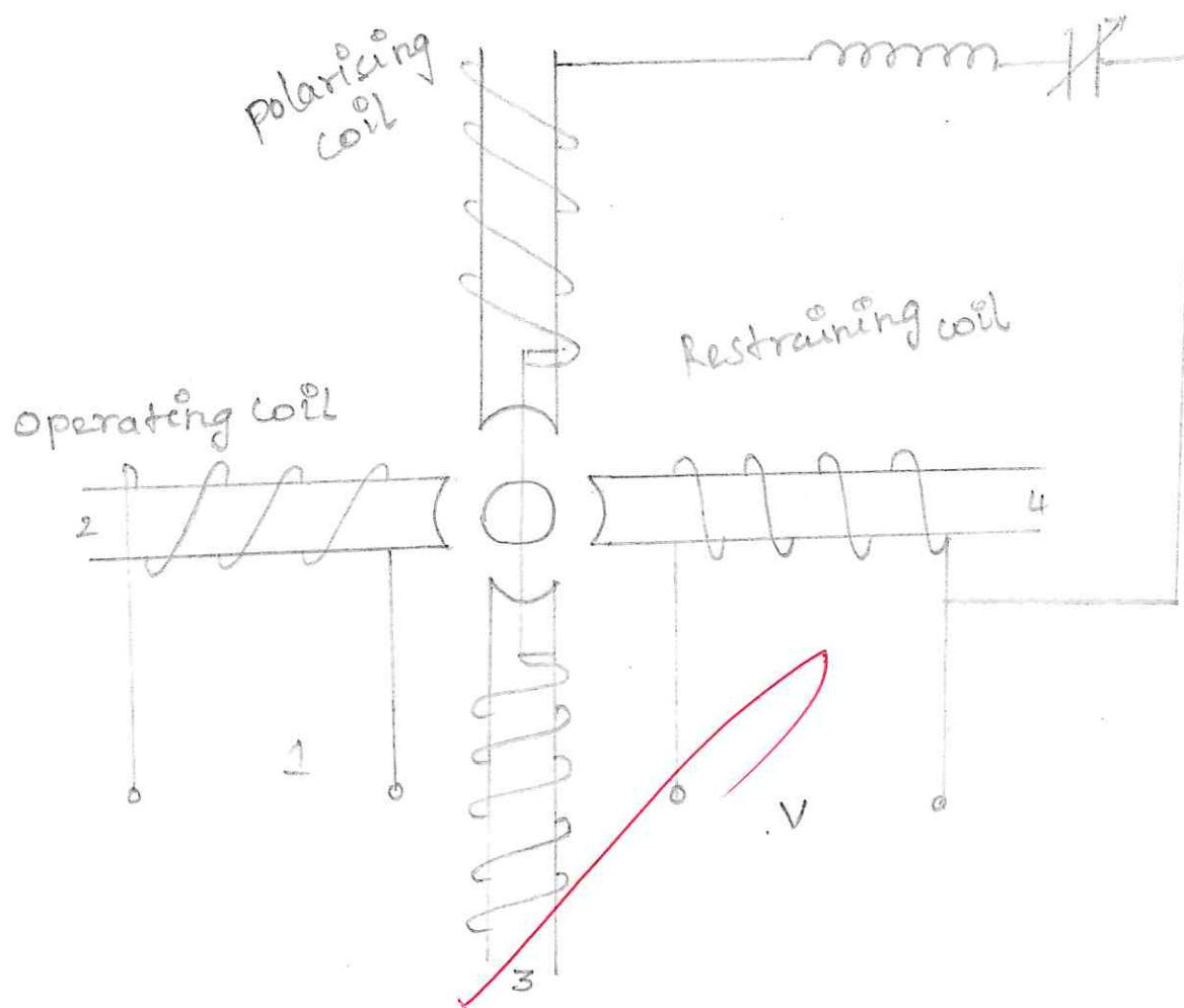
Thus an admittance relay is a voltage restrained directional relay
