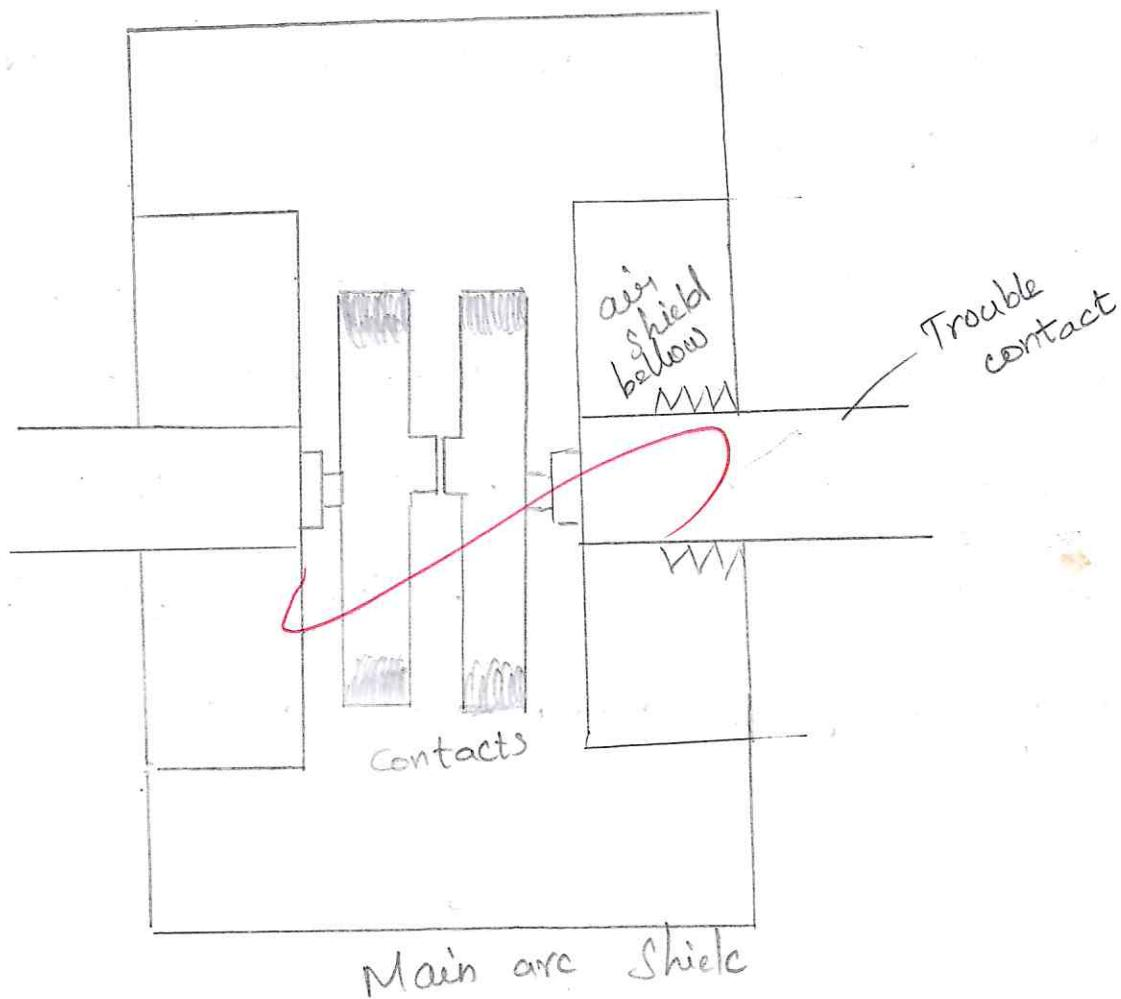
It consists of fixed contacts, moving contacts and arc shield mounted inside a vacuum change the mountain member is connected to the control mechanism by stainless steel bellows this enables the permanent sealing of the vacuum chamber of eliminate the possibility of leak
