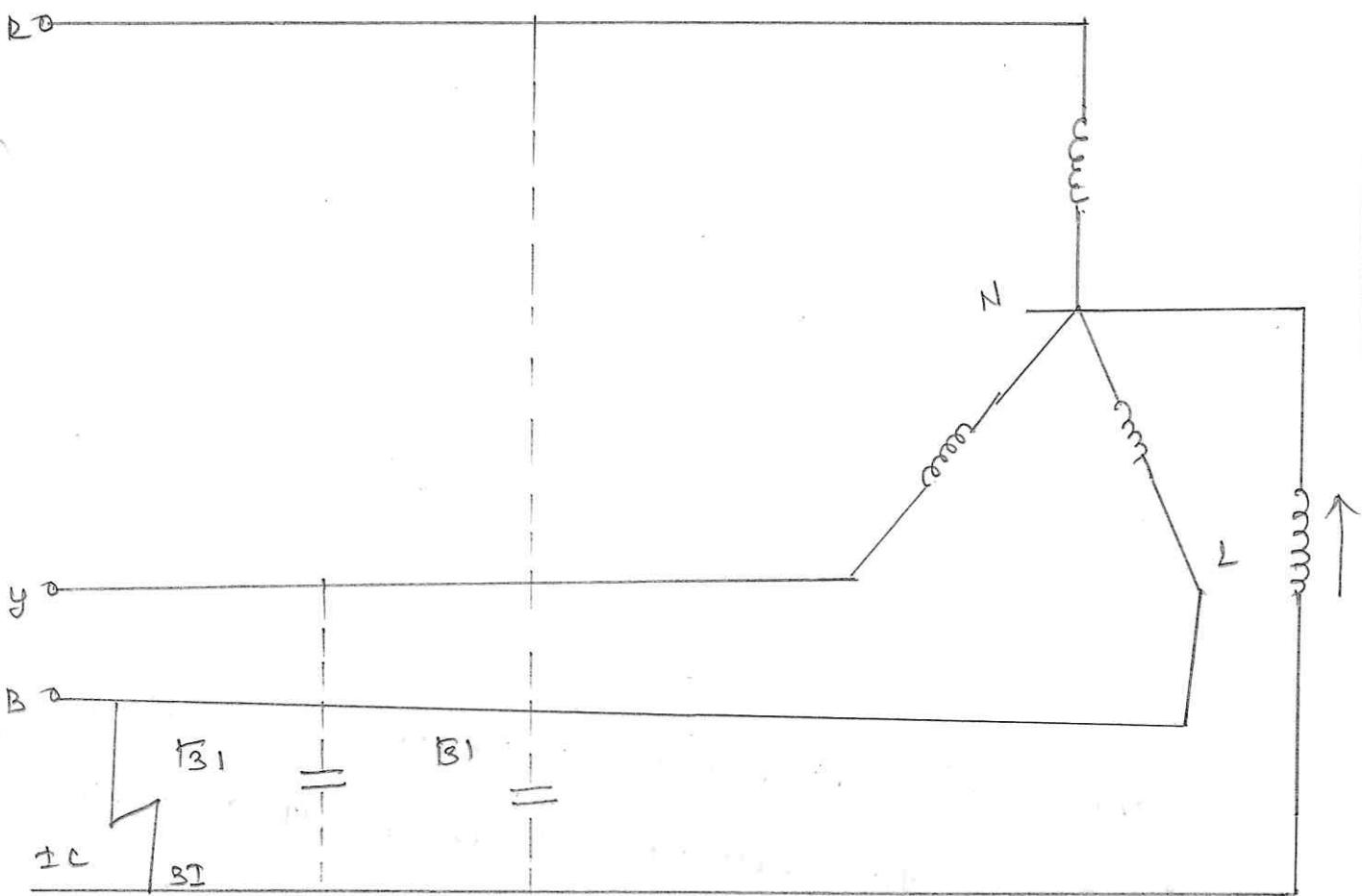
If resistance is used fault current is limited and system resistance provides the necessary phase opposition between capacitive ground current and fault current.
