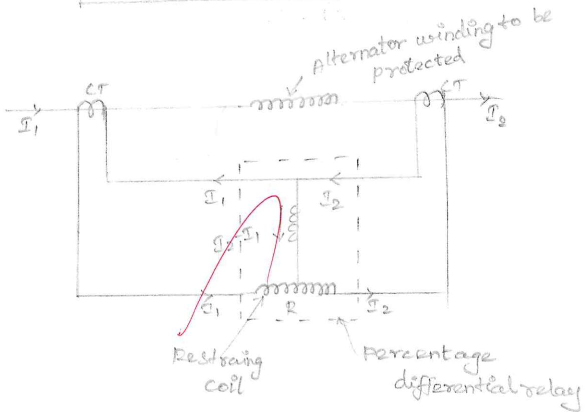
The operating coil is connected to midpoint of the restraint coil connected. The total number of ampere turns become the sum of ampere
